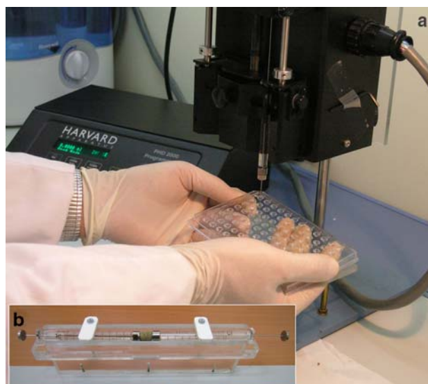
Fig. 3 Semi-automatic mesophase dispensing. a A commercially available PHD Programmable 2000 pump, from Harvard Apparatus, adapted to dispense the sample vertically. When the automatic program is adjusted to dispense aliquots up to 250 nl of cubic phase, two plates can be set-up with only one 50- \mu l-syringe load. Alongside the pump controller, a humidification system (Honeywell, model V5100N) is set to avoid the dehydration process of the protein–lipid sample. b The two syringes (50 \mu l each) mixer (Cheng et al. 1998) mounted on the homemade mixer holder
